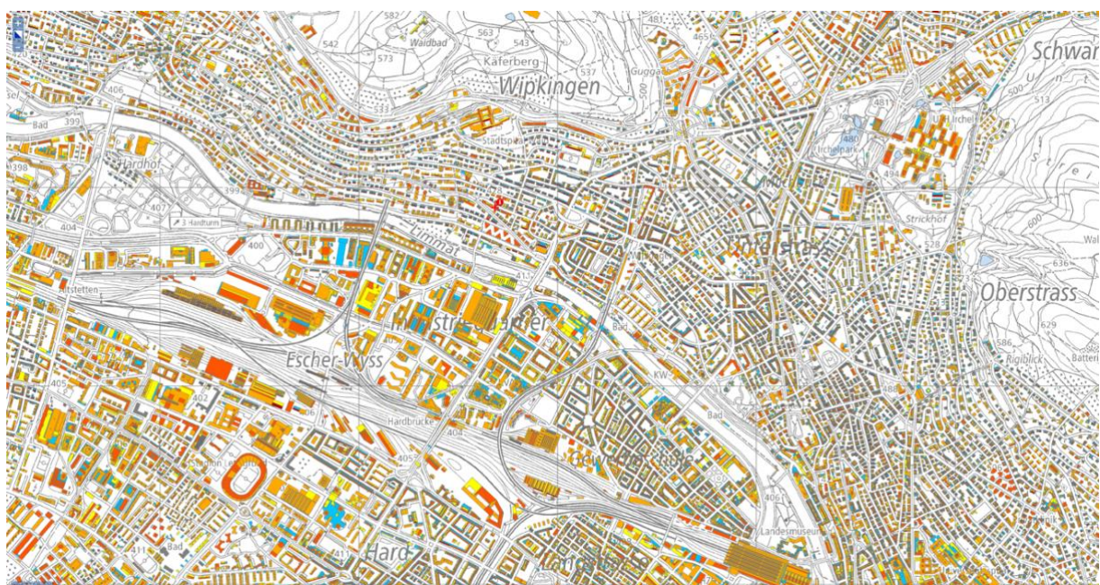
Figure 9 Suitability zones for solar energy in Zurich (partial area shown).
